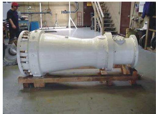
The skidded Venturi rehabilitated and ready for return to service. The annular chambers at entrance and throat were thoroughly descaled and cleaned of blockage similar to figure #1 above.
