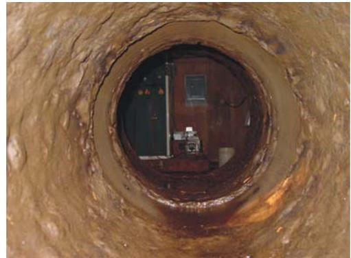
Viewing upstream through throat section of BIF Venturi meter prior to Primary Flow Signal, Inc. rehabilitation work. Note scaling, corrosion, and substantial deterioration of interior geometry that can occur in Venturi meters in service four or five
