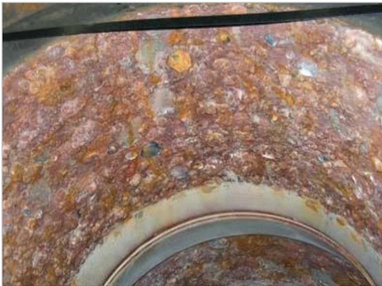
*Accuracy of Venturi flow meters can be impacted by corrosion and internal build-up.*
