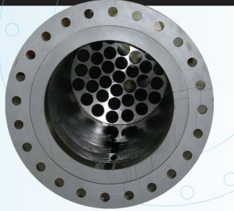
The **PFS PTC-6 ASME flow nozzle** provides the high precision needed for the testing of steam turbines under ASME PTC-6 2004 Performance Test Code. The PTC-6 ASME integrates flow conditioners for added accuracy, and diffuser cones to reduce downstream pressure loss, and also provides flanged-end PTC6-PTFFR and weld-in PTC6-PTWWR style nozzles.
